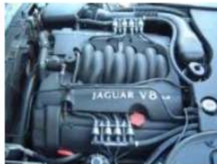
LPG injectors and pipe work
