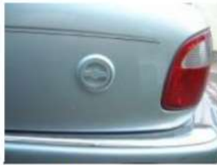
A typical LPG filler connection
