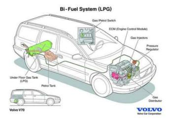
The LPG tank is usually located in the rear of the vehicle. This can be in the boot, in the spare wheel well or on brackets underneath the vehicle. Tanks are either cylindrical (as shown above) or Toroidal (dough-nut shaped to fit in the spare wheel well.
